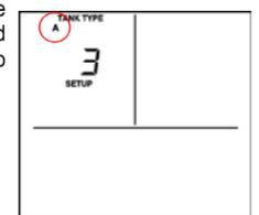
**SETUP 3 – Setting the tank type** Select Tank Type i.e. A, B, or C, using  $\Delta/\nabla$  to match the Type you noted from above. Press **ENTER** to save.
