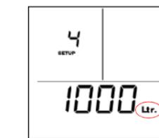
**SETUP 4 – Setting the tank capacity (Ltr)** Refer to the chart above for nominal capacity and adjust the amount in Litres displayed using  $\Delta/\nabla$ . Press **ENTER** to save.
