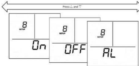
**SETUP should now be complete.** Press **SETUP** to exit and progress to STEP 3. On exiting SETUP mode the Tekelek EcoOil Monitor temporarily displays 'CALC'.
