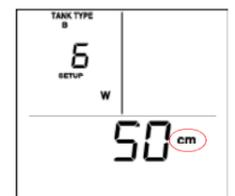
**SETUP 6 (Type B & C tanks only) - Setting the tank width (cm)** Refer to the tank chart above for the width and adjust the amount in cm displayed using  $\Delta/\nabla$ . Press **ENTER** to save.
