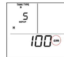
**SETUP 5 – Setting the tank height (cm)** Refer to the chart above for tank height and adjust the amount in cm displayed using  $\Delta/\nabla$ . Press **ENTER** to save. Note that if Tank Type 'A' was selected, SETUP 6 will be skipped.
