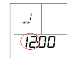
**SETUP 1 – Setting the time (hrs)** Adjust the hour displayed using  $\Delta/\nabla$ . Press **ENTER** to save.
